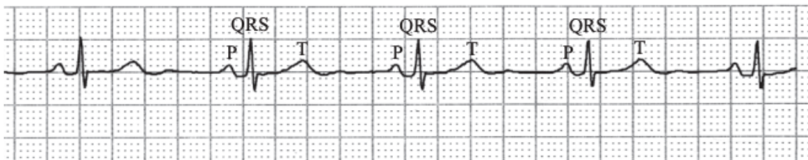
Figure 2: Typical ECG signal with annotated features [26]
